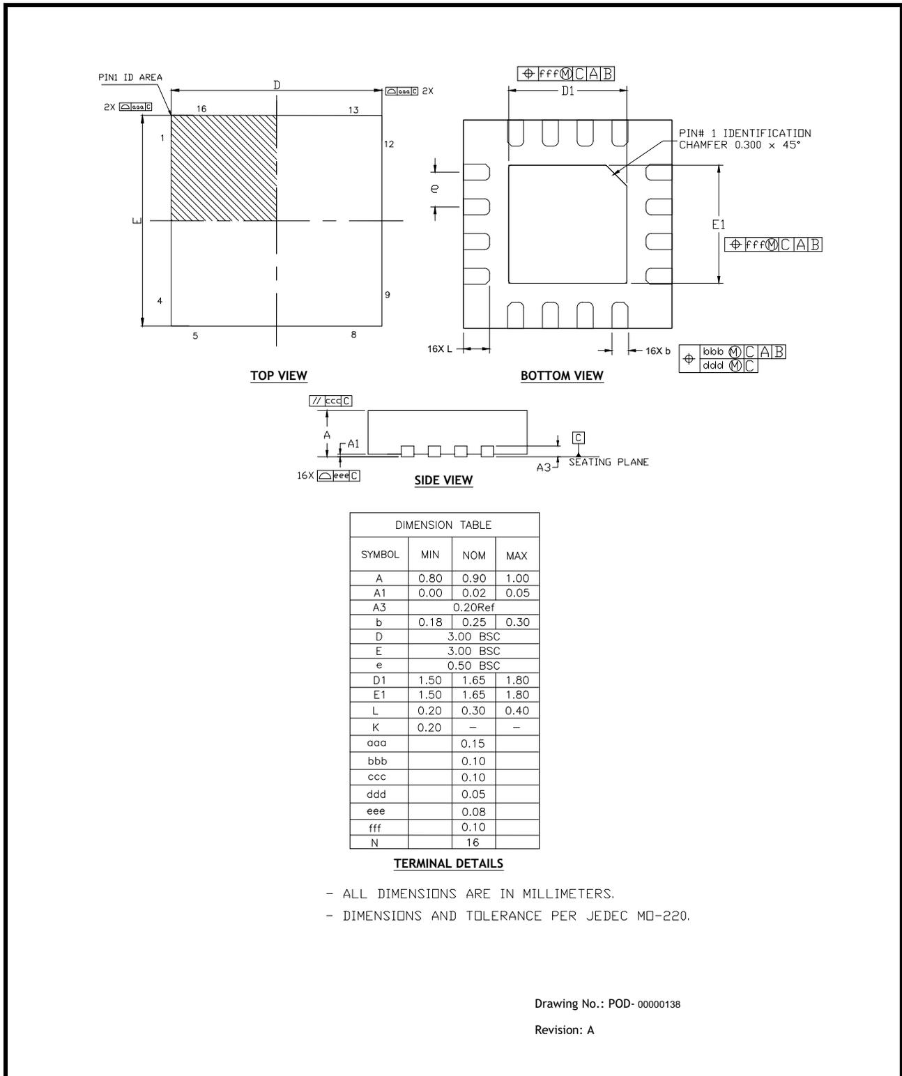
NOTE: QFN16 3x3  $\theta_{JA} = 36.4\text{ }^{\circ}\text{C/W}$ ,  $\theta_{JC} = 17.8\text{ }^{\circ}\text{C/W}$ . All values are typical.
