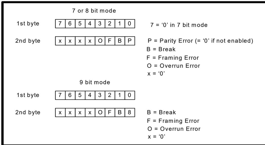
Error flags are also available from the ERROR\_STATUS register and the interrupt packet, however these flags are historical flags indicating that an error has occurred since the previous request. Therefore, no conclusion can be drawn as to which specific byte(s) may have contained an actual error in this manner.
