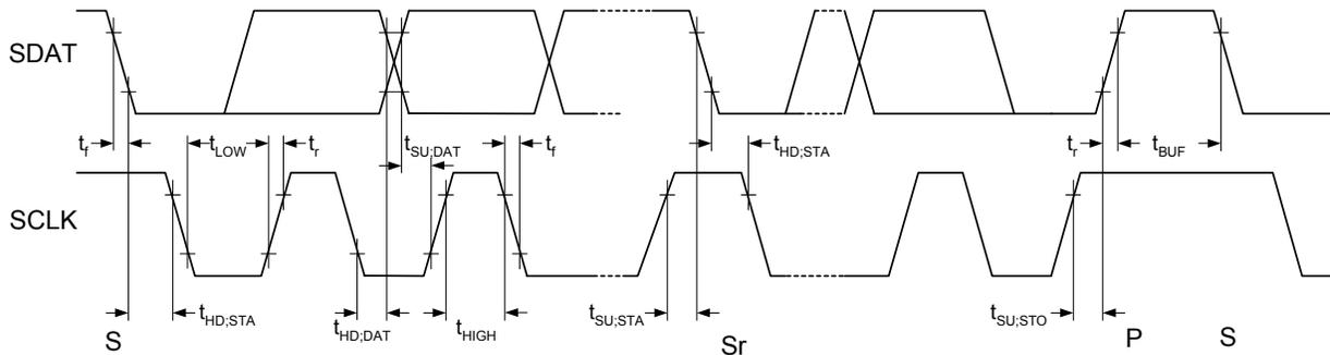
Table 16. Serial Programming Interface Timing Specifications
