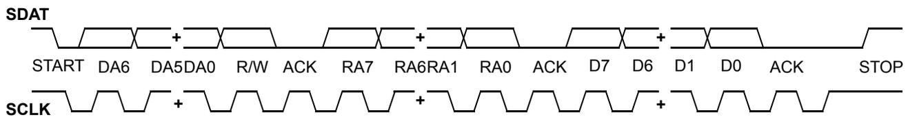
Figure 17. Definition for Timing on the Serial BUS
