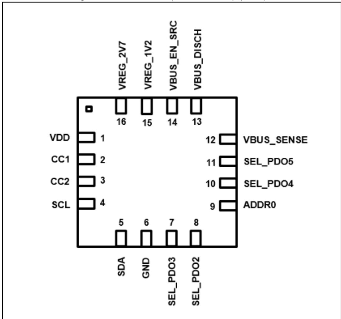
Figure 4: STUSB4710DTR pin connections (top view)
