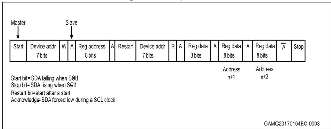
Figure 6: Write operation
