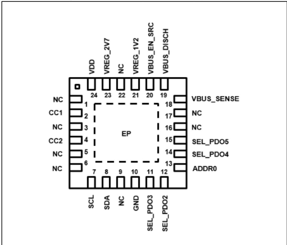
Figure 3: STUSB4710Q1TR pin connections (top view)
