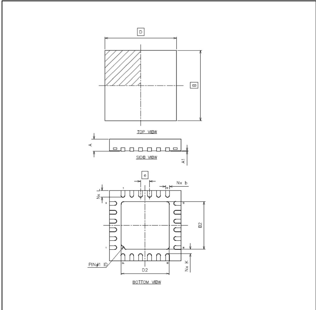
Table 17: QFN24 EP 4x4 mm mechanical data
