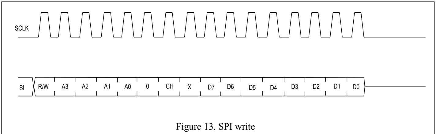
**Figure 13. SPI write**
