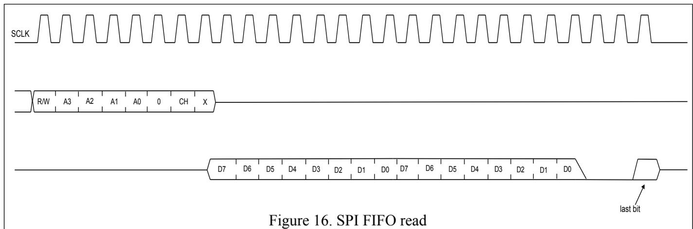
Figure 16. SPI FIFO read
