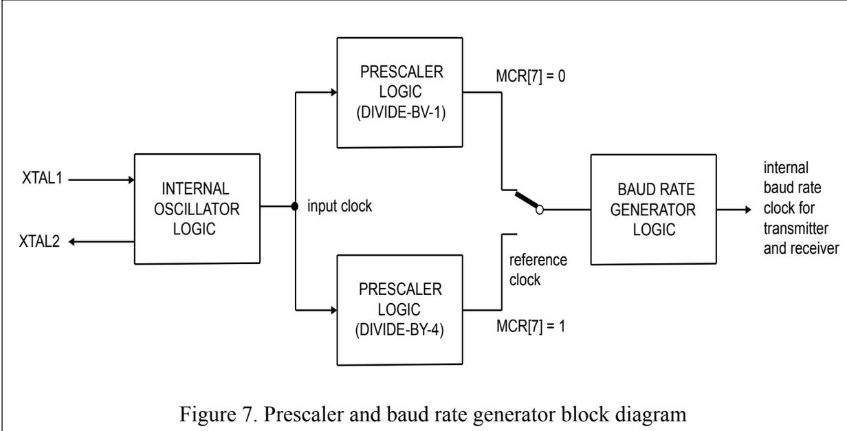
Figure 7. Prescaler and baud rate generator block diagram
