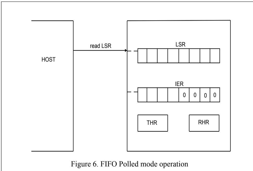
Figure 6. FIFO Polled mode operation
