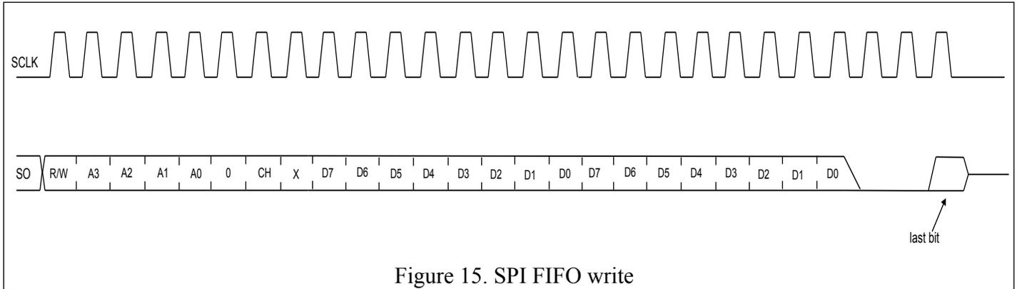
Figure 15. SPI FIFO write
