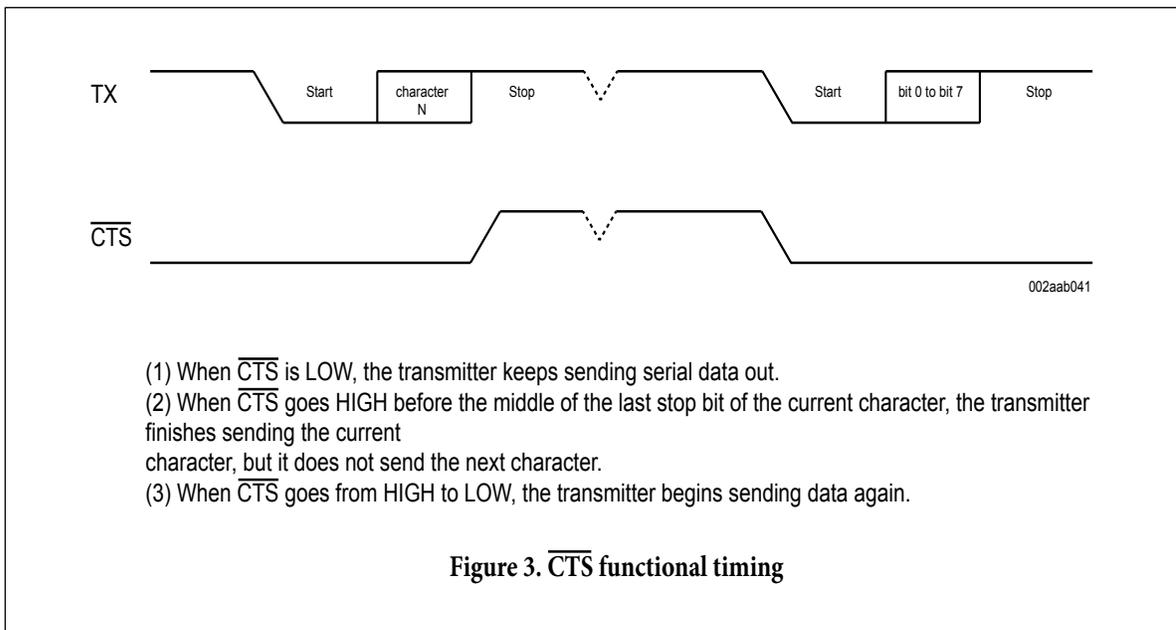
Figure 3.  $\overline{\text{CTS}}$  functional timing
