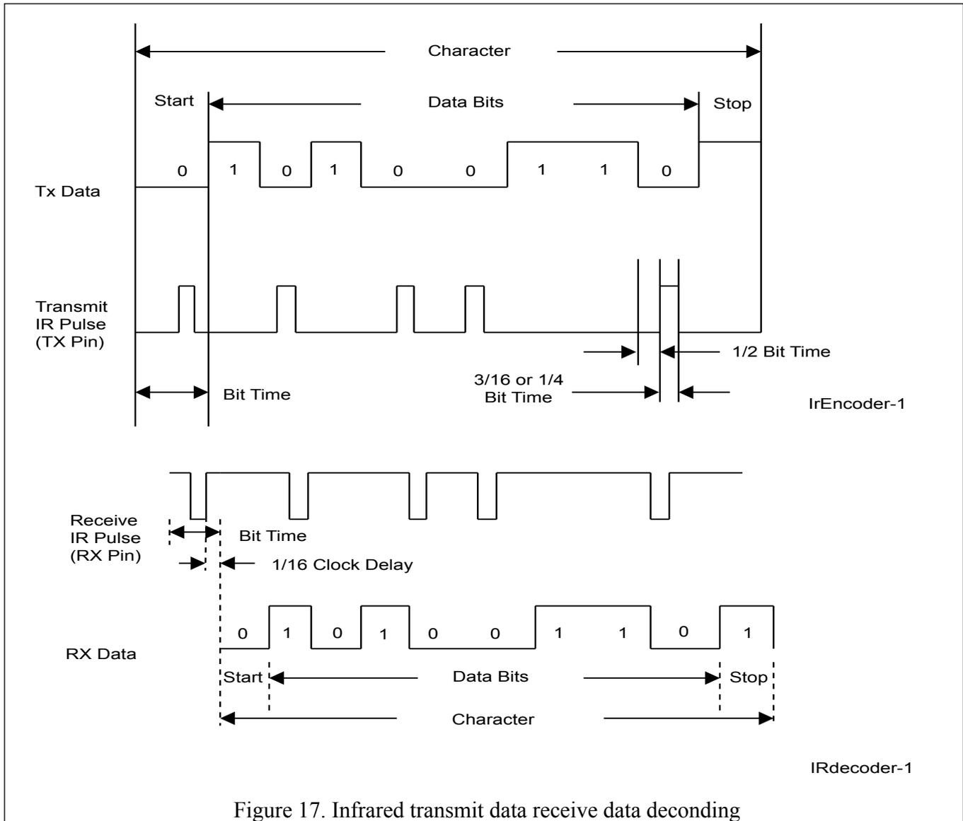
Figure 17. Infrared transmit data receive data decoding
