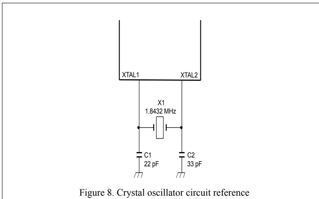
Figure 8. Crystal oscillator circuit reference
