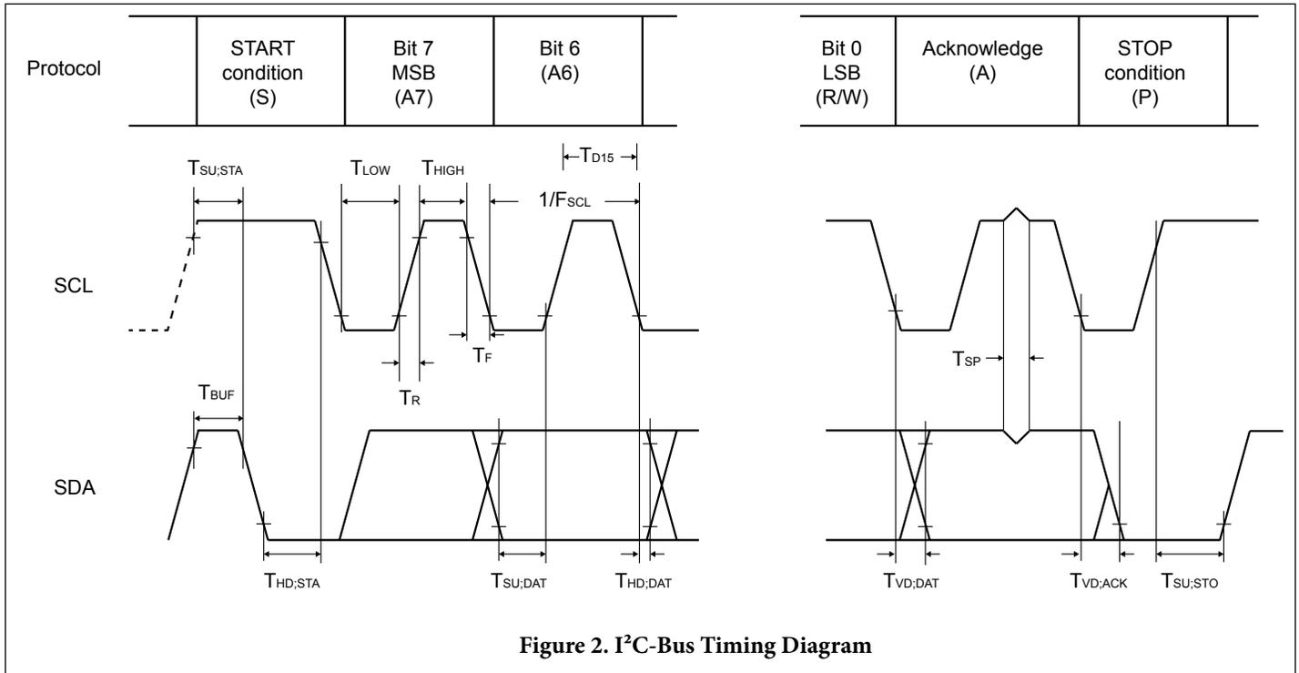
**Figure 2. I<sup>2</sup>C-Bus Timing Diagram**
