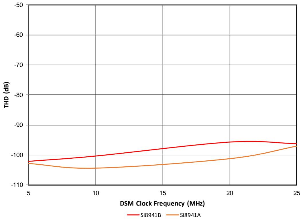
Figure 4.20. Total Harmonic Distortion vs. DSM Clock Frequency
