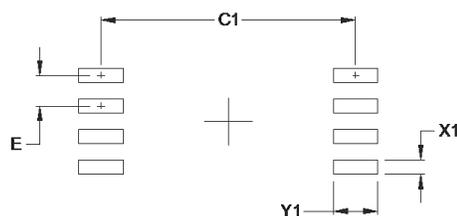
Figure 6.3. 8-Pin Wide Body Stretched SOIC Land Pattern
