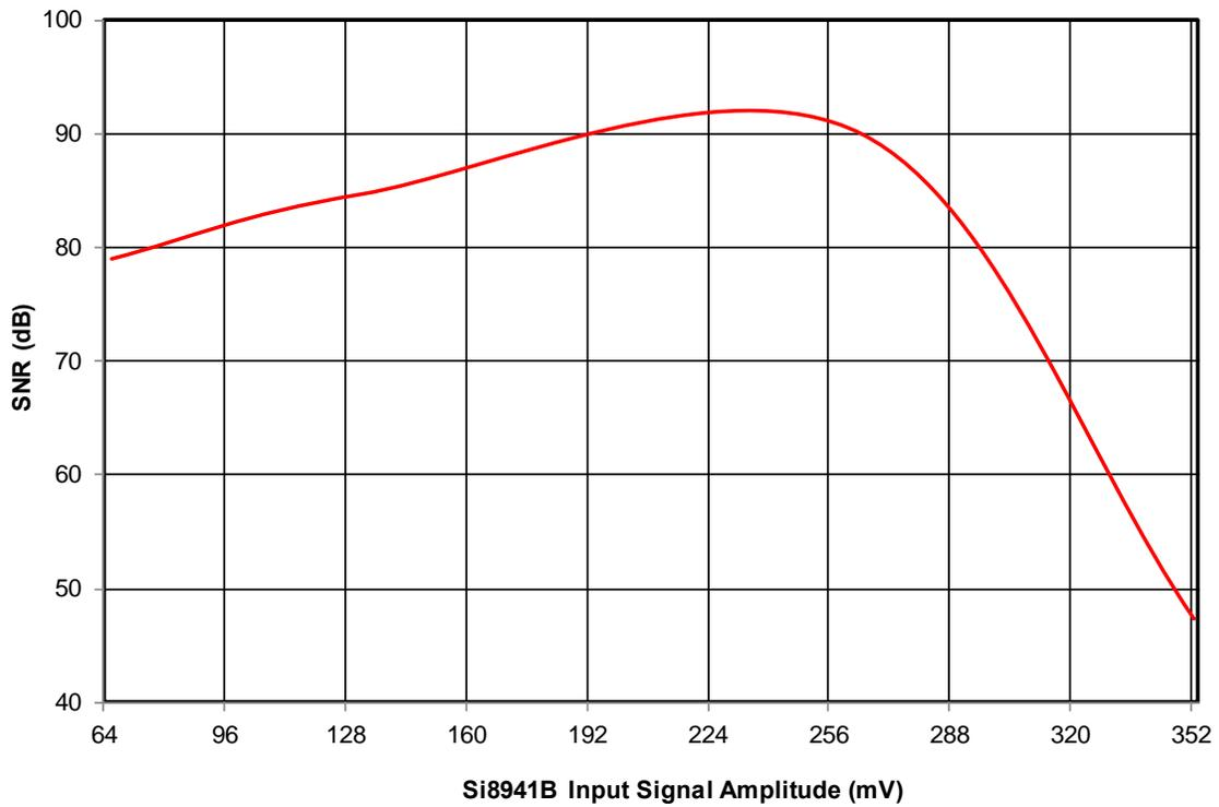
Figure 4.15. Si8941B Signal-to-Noise Ratio vs. Input Signal Amplitude
