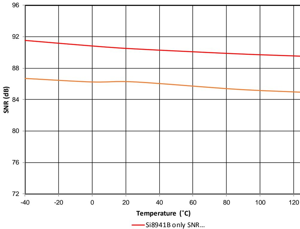
Figure 4.13. Si8941 Signal-to-Noise Ratio vs. Temperature
