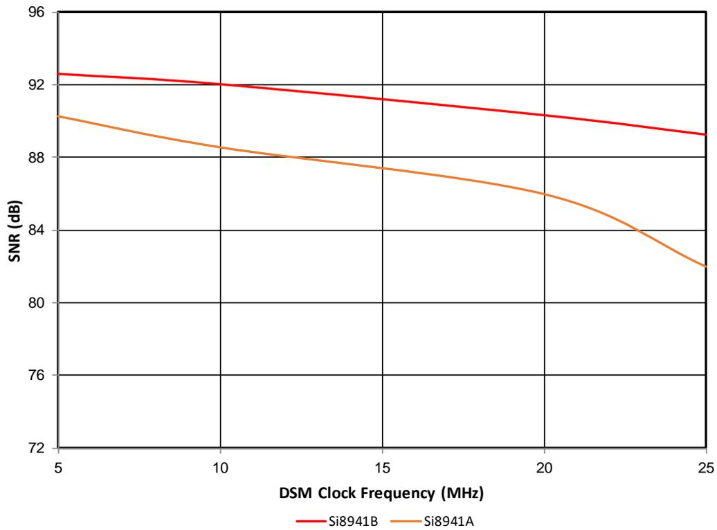
Figure 4.14. Signal-to-Noise Ratio vs. DSM Clock Frequency
