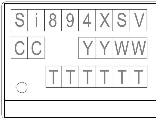
**Figure 6.6. 8-Pin Narrow Body SOIC Top Marking**
