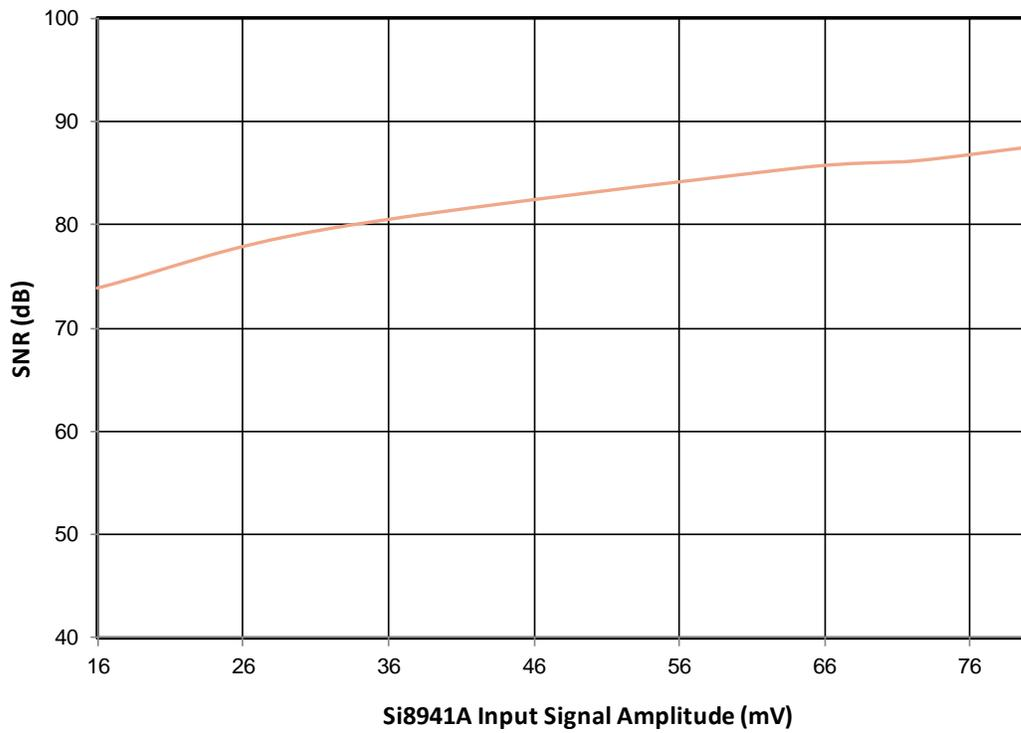
Figure 4.16. Si8941A Signal-to-Noise Ratio vs. Input Signal Amplitude
