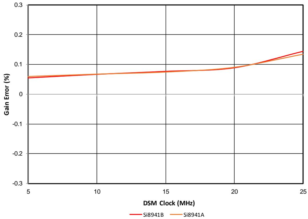
Figure 4.8. Si894x Gain Error vs. DSM Clock Frequency
