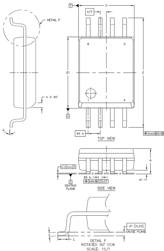
Figure 6.1. 8-Pin Wide Body Stretched SOIC Package
