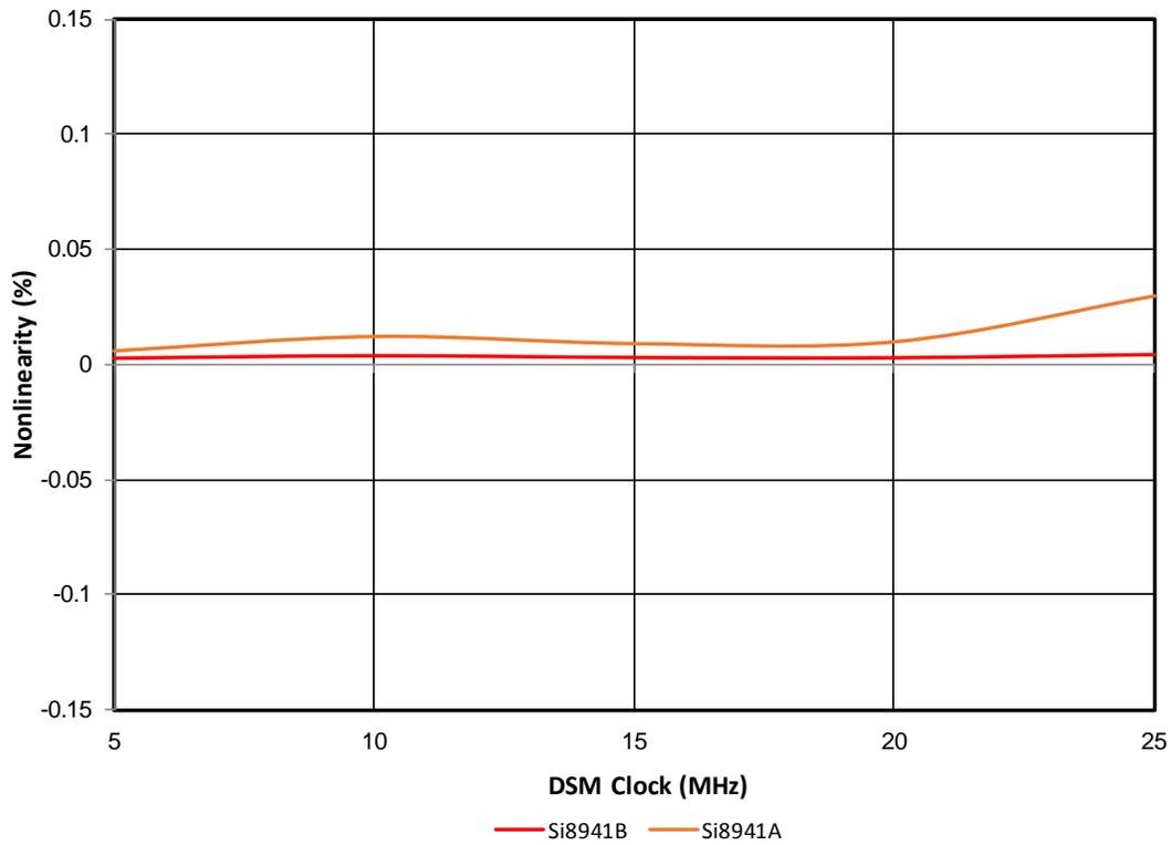
Figure 4.10. Si894x Nonlinearity vs. DSM Clock Frequency
