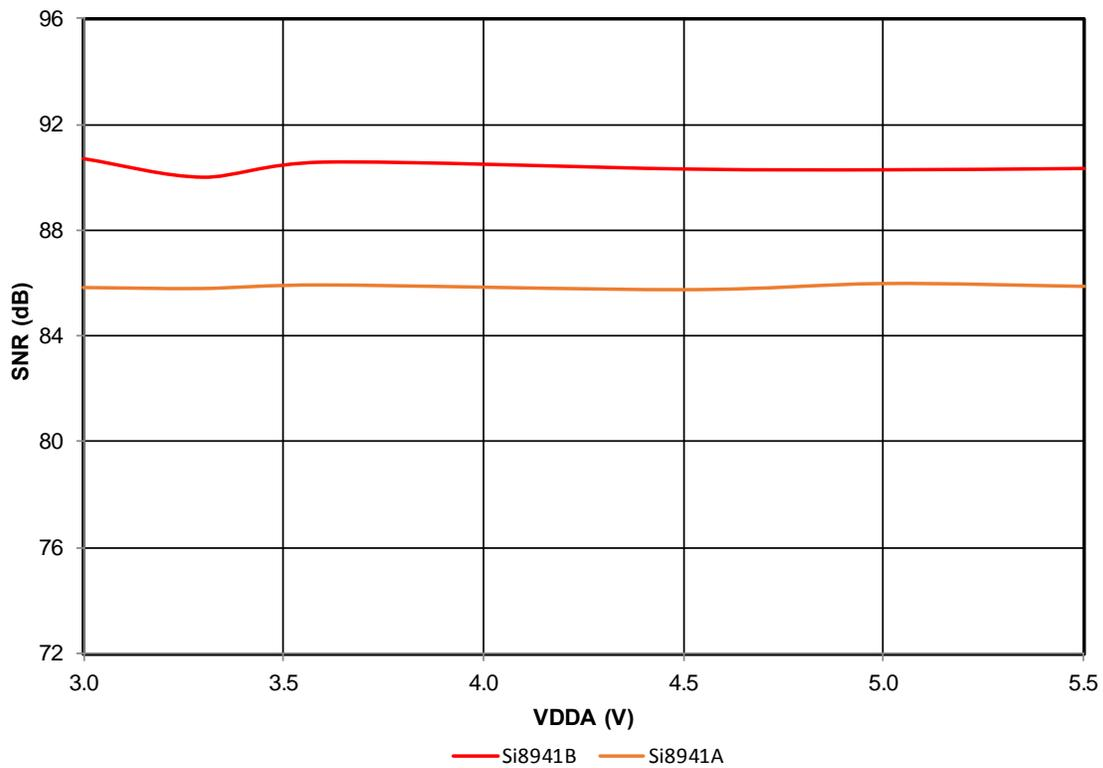
Figure 4.11. Si8941 Signal-to-Noise Ratio vs. VDDA
