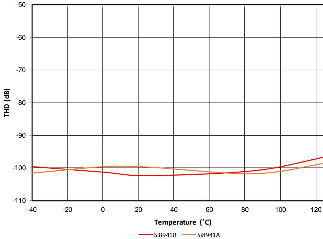
Figure 4.18. Si8941 Total Harmonic Distortion vs. Temperature
