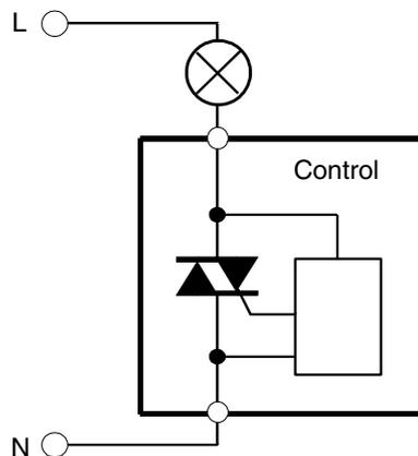
**Figure 4.** Three-wire Circuit
