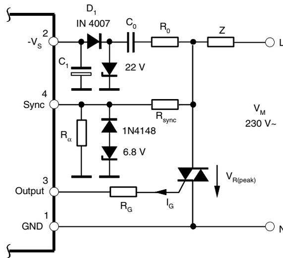
$$C_1 = 100 \mu\text{F}/35 \text{ V}$$
