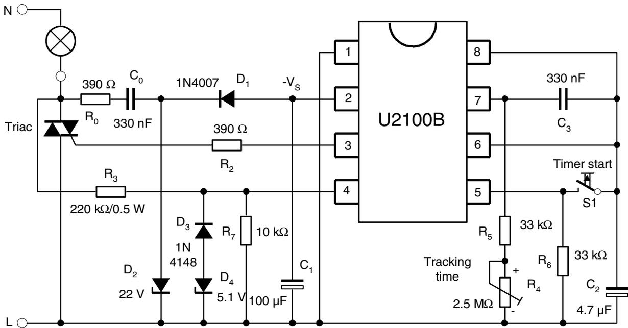
**Figure 11.** Fan Tracking Time Control 18 Seconds to 23 Minutes
