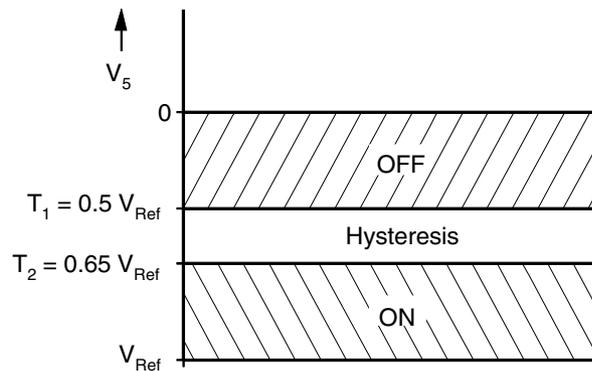
**Figure 9.** Trigger Condition, Pin 6
